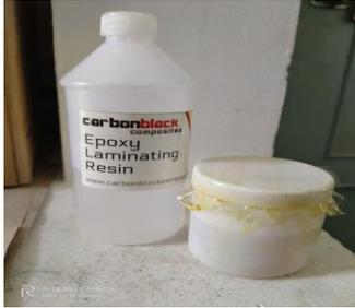
Fig. 2. Epoxy laminating resin and hardener
