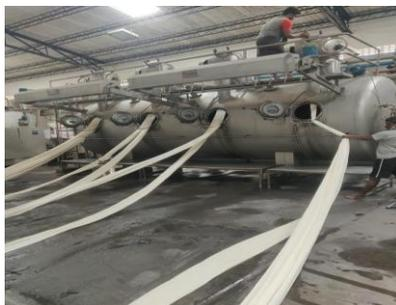
Fig. 3. High temperature high pressure soft flows dyeing machine
