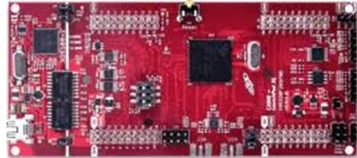
Fig. 3. TMS320F28379D microcontroller
