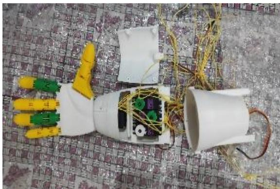
Fig. 3. Fingers are controlled by tendons actuated through servo motors placed in the forearm
