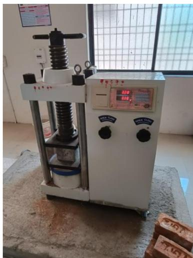
Fig. 1. Compression testing machine set up
