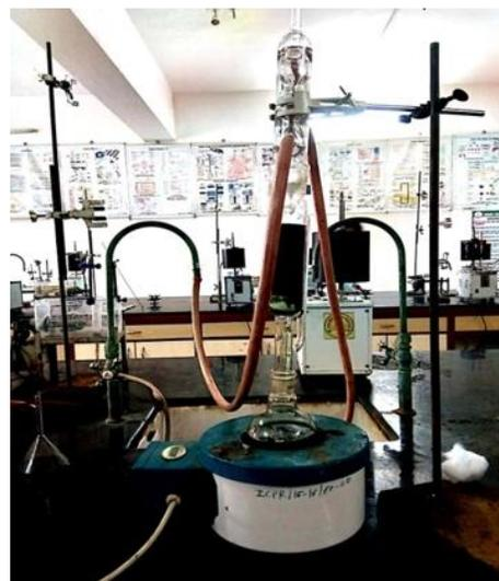
Fig. 4. Soxhlet apparatus for methanolic extraction
