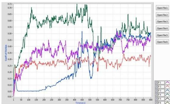
Fig. 9. Coefficient of friction at 1000rpm
