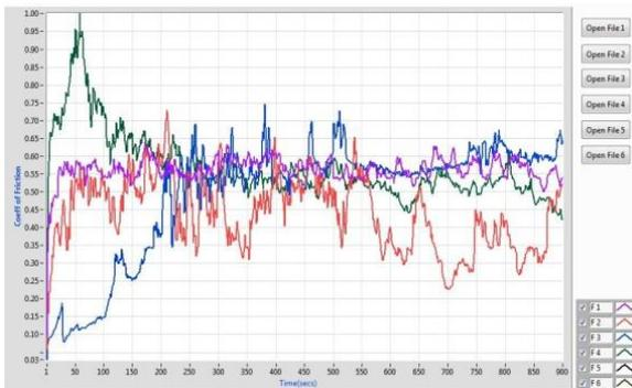
Fig. 10. Coefficient of friction at 2000rpm
