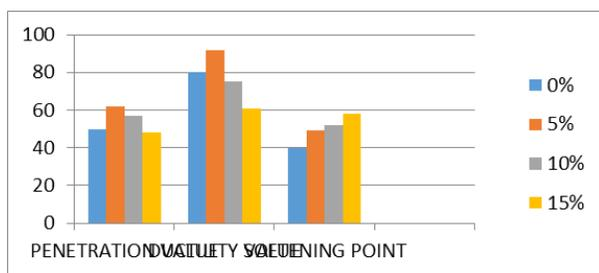
Fig. 1. Graphical representation of test results of bitumen after replacement of waste plastics
