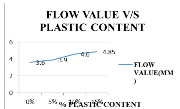
Fig. 3. %plastic in bitumen and Flow value (mm)
