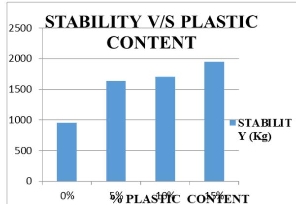
Fig. 2. %plastic in bitumen and stability (kg)
